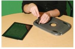
Loosen the 8 screws on the back of the case. When fully loosened, the screws will remain in the case so you don't lose them.
