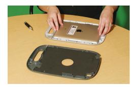
Turn the iPad face-down so its charging dock aligns with the access port near the handle of the case.
