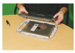
Put the back of the case on the iPad so the handle openings match.
