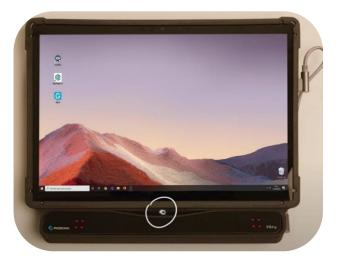
**Step 2: Calibration** is a unique set of user data that places the cursor on the screen. A successful calibration will ensure accurate and efficient tracking for the end user.
