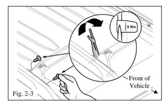
(d) Starting with the rear shoulder bolt, use the torque wrench to tighten one side of the crossbar.
