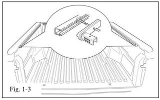
(c) Install the LH Bracket (with the WARNING label) onto the LH clamp plate threaded stud. (Fig. 1-3)
