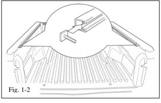
(b) Slide one clamp plate into each side rail. (Fig. 1-2)
