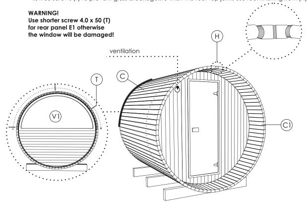
**STEP 7:** Measure steel bands (I) to ensure correct length of 500mm is acceptable. Install steel bands (I) by wrapping bands around barrel prior to connecting with bolts and nuts (U). Place steel bands evenly around barrel, covering screw heads. Measure from steel band to barrel edge to ensure the steel band is even. Cover roof with roof tape. Rub and smooth with pressure to ensure adhesion. Install interior aspen roof trim (O) with 4.0 x 35 (P) screws.
