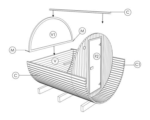
**STEP 6:** Continue placing body staves (C,C1) tightly on both sides of the sauna using rubber mallet, while fixing body staves on the front panel with 4.2 x 70 screws (N) and rear window panel (V1) with 4.0 x 50 screws (T) to prevent glass breakage...To finish the roof top joint, use roof finishing item (H).
