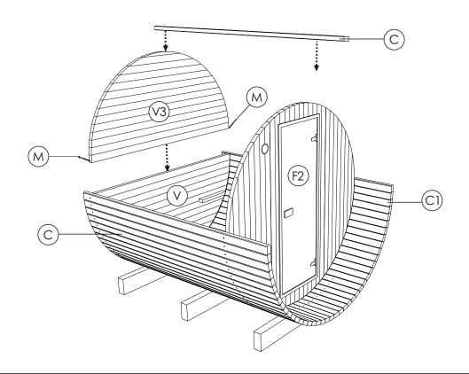
**STEP 6:** Continue placing left and right body staves (C, C1) tightly on both sides of the sauna using rubber mallet, while fixing body staves with 4.2 x 70 screws(N). To finish the roof top joint, use top stave (H).
