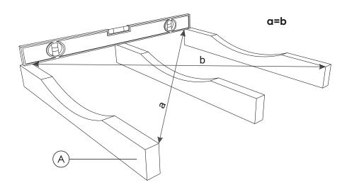
STEP 2: Place the support cradles (A) on level site. The middle support cradle will have no dowel. Carefully level for better stability. Place the center stave (B) on wooden dowels embedded in outer support cradles (A). Fix the center stave (B) with screw 4.2x70 (N).
