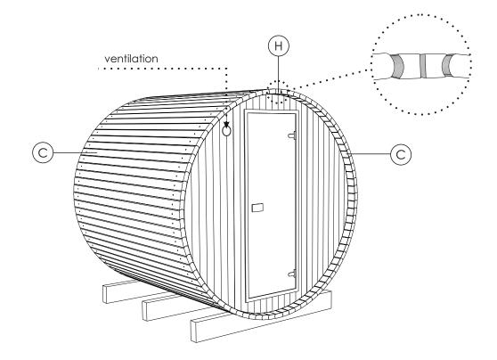
**STEP 7:** Measure steel bands (I) to ensure correct length of 100mm is acceptable. Install steel bands (I) by wrapping bands around barrel prior to connecting with bolts and nuts (U). Place steel bands evenly around barrel, covering screw heads. Measure from steel band to barrel edge to ensure the steel band is even. Cover roof with roof tape. Rub and smooth with pressure to ensure adhesion. Install interior aspen roof trim (O) with 4.0 x 35 (P) screws.
