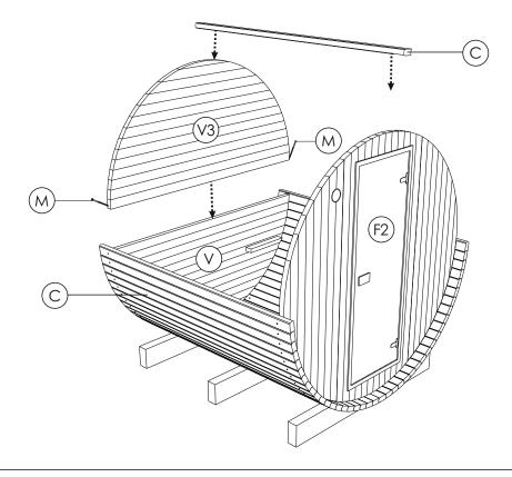
STEP 6: Continue placing body staves (C) tightly on both sides of the sauna using rubber mallet, and fixing body staves with screws 4.20x70(N). To finish the roof top joint, use roof finishing item (H).
