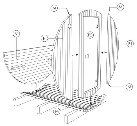
STEP 5: Place body staves (C) until the halfway point. Place upper rear panel (V3) on bottom rear panel (V), fix by 2 screws 5.0 x 120 (M). Bind panels (F2; V3)together by temporarily placing one or two body stave (C) on top of them.
