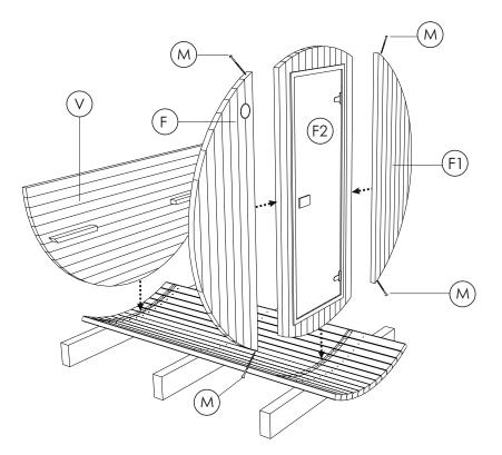
**STEP 5:** Place body staves (C,C1) until the halfway point. Place rear panel with panoramic window (V1) on bottom rear panel (V), fix by 2 screws 5.0 x 120 (M). Bind panels (F2; V1) together by temporarily placing one or two body stave (C) on top of them.
