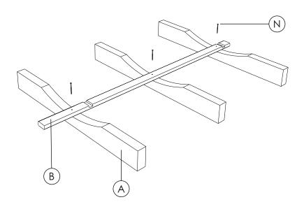
**STEP 3:** Place 6 sauna body staves (C,C1) to each side of the center stave (B) and fix with screws 4.2 x 70 (N). Body staves (C) are left and right sided. Be sure to align the panel groove on every next body stave.
