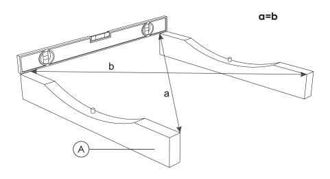
**STEP 2:** Place the center stave (B) on wooden dowels embedded in support cradles (A). Fix the center stave (B) with screw 4.2x70 (N).
