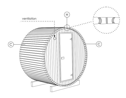
STEP 7: Measure steel bands (I) to ensure correct length of 100mm is acceptable. Install steel bands (I) by wrapping bands around barrel prior to connecting with bolts and nuts (U). Place steel bands evenly around barrel, covering screw heads. Measure from steel band to barrel edge to ensure the steel band is even. Cover roof with roof tape. Rub and smooth with pressure to ensure adhesion. Install interior aspen roof trim (O) with 4.0 x 35 (P) screws.
