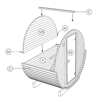
**STEP 6:** Continue placing body staves (C) tightly on both sides of the sauna using rubber mallet, and fixing body staves with screws 4.20x70(N) . To finish the roof top joint, use roof finishing item (H).
