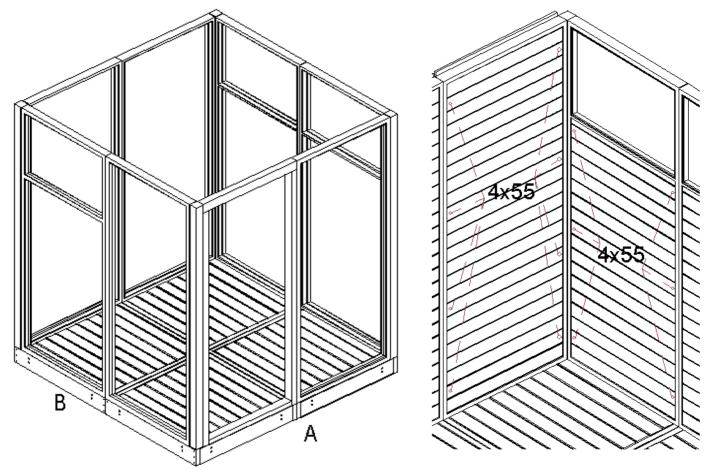
4. Install the wall elements with 4x55mm screws. The higher elements (9) with eight screws, and the lower elements (10) with six screws.
