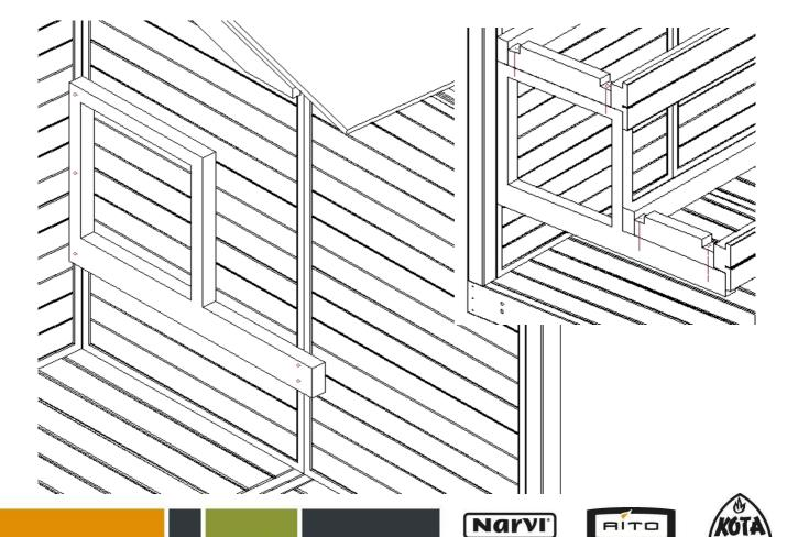
14. Install the rail (30) to the sauna bench frame with two 5x70mm screws at both ends. Fasten the screws from the frame to the rail.
