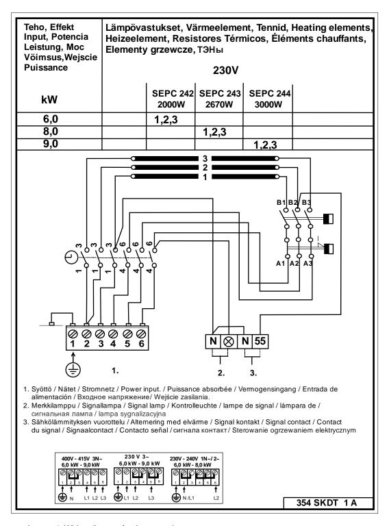
Image 4 Wiring diagram for the sauna heater
