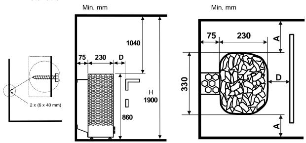
Image 2 Safety clearances distances, minimum dimensions (mm)
