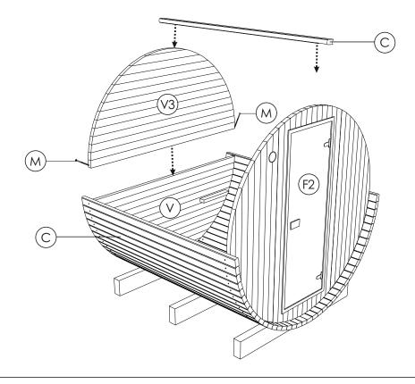
STEP 6: Continue placing body staves (C) tightly on both sides of the sauna using rubber mallet, and fixing body staves with screws 4.20x70(N). To finish the roof top joint, use roof finishing item (H).
