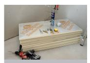
1. The installation of Kingspan Sauna-Satu® is easy and efficient. You only need a carpet knife, fasteners, foam sealant (OCF) and aluminum
