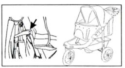
1.To open stroller: release the folding hook as the picture shown, lift the handlebar, unfold the stroller and make sure both joints locked.
