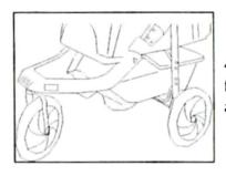
**4.**To attach footboard: attach footboard position to bottom and tighten screws.
