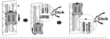
Loosen the Thumbscrew on VESA Bracket (A) to separate into three parts: Bracket (A1), VESA
