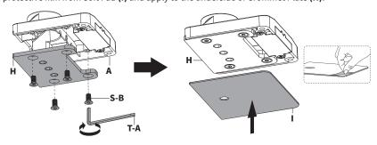
Position Base **(A)** over grommet hole in desk. If there is no existing grommet hole, drill a 0.375" (10mm) hole through the desktop in the desired mounting position.
