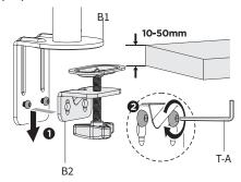
For thicker desktops (40-85mm), disassemble Lower Clamp (B2) using a Phillips screwdriver as shown below. Flip the L-bracket over and reassemble. Then re-attach Lower Clamp (B2) to Upper Clamp (B1) and tighten the screws using 4mm Allen Wrench (T-A). Tighten the clamp assembly to the desktop.
