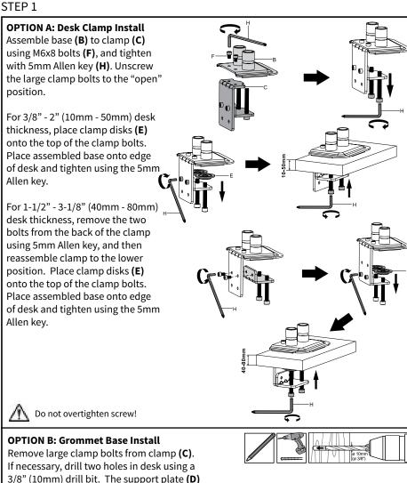
3/8" (10mm) drill bit. The support plate (D) may be used as a drill guide. Secure base (B) to desk using clamp bolts with support plate (D), and tighten using 5mm Allen key (H). NOTE: Grommet option will fit a desk thickness of 3/8" - 1-3/4" (10mm - 45mm).
