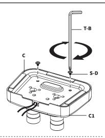
Disassemble Lower Clamp (F) using the Phillips end on 5mm Allen Wrench (T-B).
