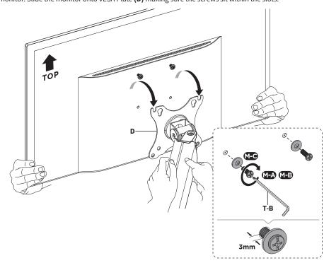
Tighten the top two screws and install the remaining Screws (M-A or M-B) and 5mm Washers (M-C) using the Phillips end on 5mm Allen Wrench (T-B).
