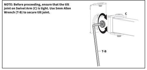
Slide VESA Plate (**D**) with adapter and tablet onto the head of Swivel Arm (**C**). Install the M6 Security Nut (**S-B**).
