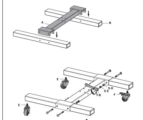
**NOTE:** You will need an adjustable wrench or a 17mm (11/16") wrench to tighten the Casters. Wrench included is intended to for this purpose.
