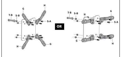
Then use Screws (M-A thru M-D) along with Washers (M-E, M-F) to secure VESA plate assembly to the back of your television. Make sure the "VIVO" logo is right side up. For a curved television, Spacers (M-G) may be required.
