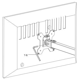
To level the monitors, remove the security nut and turn the bolt with 3mm Allen Wrench (T-A) to raise or lower the monitor. Replace nut after the adjustment.
