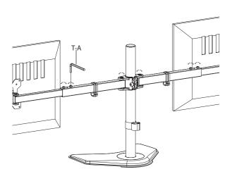
Manage cables and store Allen Wrenches in Pole Cable Clip (G) for future use.
