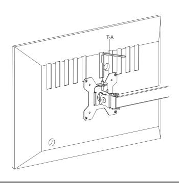
Use 3mm Allen Wrench (T-A) to adjust joints if needed.
