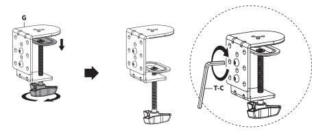
Install Lower Pole (B) to Clamp (G) using M6x16mm Screws (S-B) and 3mm Allen Wrench (T-A). Attach Clamp (G) to desktop.
