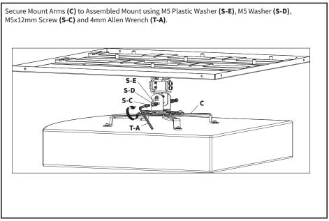
Adjust angle and rotation of projector if desired by loosening screws on Assembled Mount using 4mm Allen Wrench **(T-A)**.
