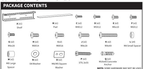
WARNING: CHOKING HAZARD small parts-not for children under 3 years. Adult supervision is required.DO NOT INSTALL INTO DRYWALL ALONE. VERIFY YOUR WALL CONSTRUCTION. USE WOOD STUDS TO MOUNT.
