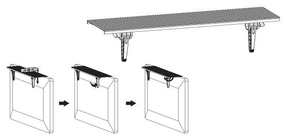
Place the shelf onto the top of the TV with the front of the shelf hooked over the edge of the TV. Place a level on the shelf, then adjust the legs to touch the back of the TV while holding the shelf level. Tighten the knobs, then place the anti-slip rubber pad on the surface of the shelf.
