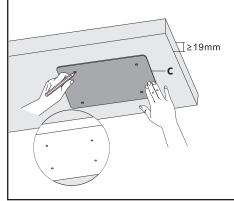
Use a 5/32 (4mm) drill bit to drills holes 0.6" (16mm) deep. Screw in ST5.5x19mm Screws (**S-B**) inline with the keyhole slots on the mount, using a phillips head screwdriver, leaving 1/8" (3mm) of space between the desktop and the screw head.
