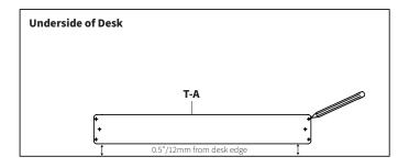
Drill 3/8" (10mm) deep holes using a 1/8" (3mm) drill bit. Mount keyboard tray assembly using M5x14mm Screws **(S-B)** and a Phillips screwdriver.
