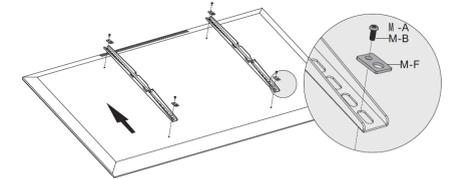
Secure mounting brackets (**B**) to the TV using metal spacers (**M-F**) and bolts (**M-A**, **M-B**, **M-C**), depending on the size of the mounting holes on the back of the TV. If the bolts are too long, spacers (**M-G**, **M-H**) may be required as shown in diagram.
