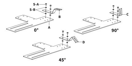
Install compatible Foot (B, C, D) for your passenger seat's left bolt to the threads on Connecting Bracket (L) using M6 Nuts (S-C), M6 Washers (S-B), and Wrench (T-B). Please note, based on your passenger seat's floor bolts, you may need a different foot than what was used above.
