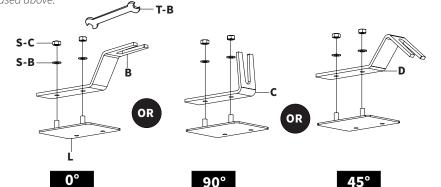
M6 Washers **(S-B)**, and a Phillips screwdriver. Align the left foot with the left seat bolt on the passenger seat. Adjust the right foot to match up with the right bolt on the seat and tighten M6x10mm Screws **(S-A)**.
