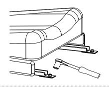
Slide the left foot under the left seat bolt and the right foot under the right seat bolt. Adjust the placement as needed and re-tighten bolts.
