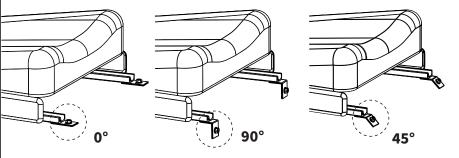
Attach the appropriate foot for the passenger seat's left bolt [0° Foot (B), 90° Foot (C), or 45° Foot (D)] to the left underside of of Base (A) using M6x10mm Screws (S-A) M6 Washers (S-B), and a Phillips screwdriver.
