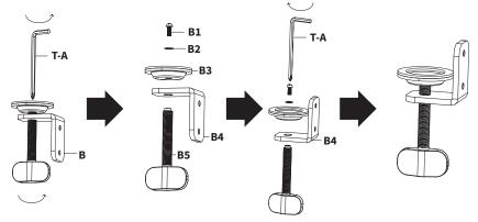
\*Follow steps below for to mount Lower Clamp (B) to Upper Clamp (A) based on your specific mounting surface thickness.
