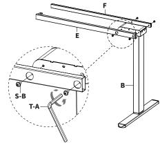
Slide crossbars of third leg assembly onto the existing assembly to form a corner frame shape. These will be secured in a later step.
