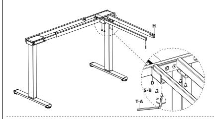
Assemble Inner Crossbar (F) and Outer Crossbar (E) to remaining Motorized Leg (B) using M6x11mm Screws (S-B) and 5mm Allen Wrench (T-A).
