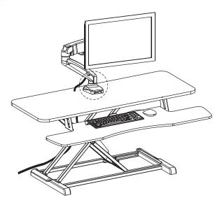
To utilize this feature, your will need to remove the plug from the top surface of the riser. Secure your mount using a grommet mounting method, using the hardware and assembly steps from your monitor mount.
