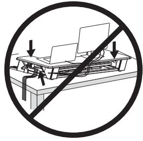
Follow the cable routing instructions to avoid the potential to pinch cables.
