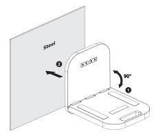
Mounting Surface Must Be At Least 1mm Thick Before mounting, ensure intended surface is at least 1mm thick.
