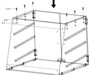
Place Front Panel (E) on the angled front edge of the display case and insert M5x15 Screws (S-A) into the pre-drilled holes and then slide Lock Washers (S-B) onto M5x15 Screws (S-A) and secure with M5 Nuts (S-C). Gently tighten with an adjustable wrench until the nut is snug. Do not over tighten.
