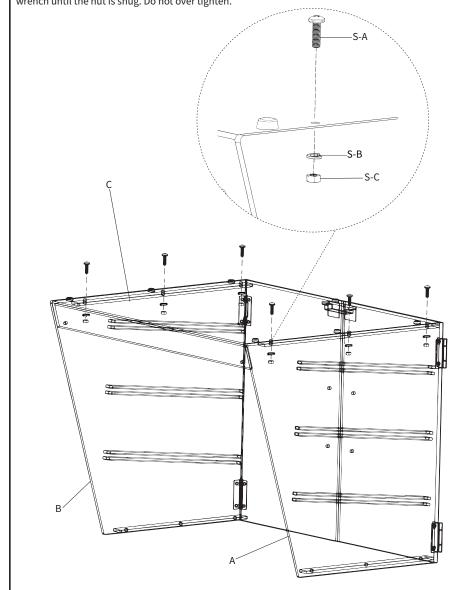
Flip the display case over and align Top Panel (**D**) with the pre-drilled holes. The bent side of this piece will be at the front of the case. Insert M5x15 Screws (**S-A**) into the pre-drilled hole and then slide Lock Washers (**S-B**) onto M5x15 Screws (**S-A**) and secure with M5 Nuts (**S-C**). Gently tighten with an adjustable wrench until the nut is snug. Do not over tighten.
