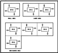
The CM-12 should be installed on the ceiling in nearly all applications. This is especially important when the air cleaner is used for smoke control. Visible smoke contains very small particles, so small in fact, that they are not noticeably affected by gravity. Smoke usually rises to the ceiling and hangs there.
