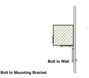
L-Brackets should be 6" from the ends of the unit
