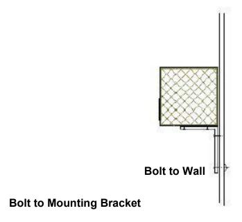
L-Brackets should be 6" from the ends of the unit
