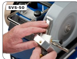
SVS-50 Multi Jig For skewes of any shape, even with an oval section.
