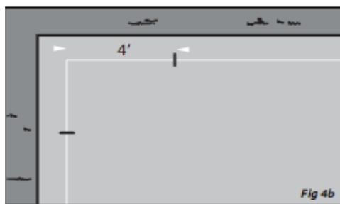
**b)** Measure 4 feet (or 8 feet) down the perpendicular string line and make a mark (Fig 4b - Line a-c).
