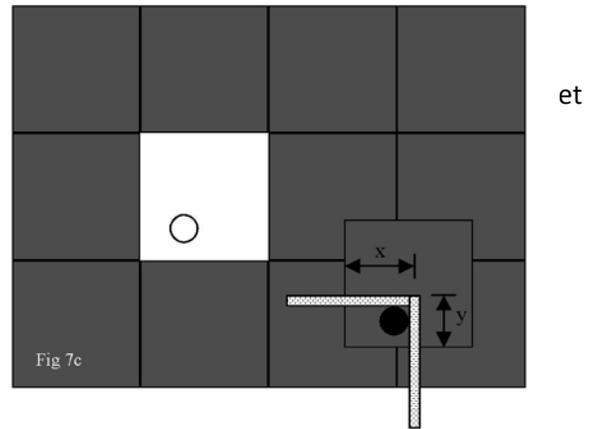
5. Place your template into the center of the “square” and mark the perimeter of the template. You are now ready to make your cut (Fig 7c).
