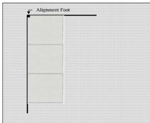
The tiles are designed to fit as tightly as possible to the adjacent tile. Some force may be required to achieve the tight fit. This is normally done by using a rubber mallet or the heel of your foot to align the tiles and insure tight fit.
