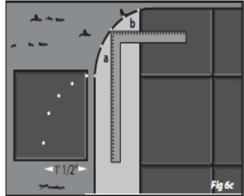
**3.** After the measurements have been transferred onto the tile to be cut, connect the markings using a flexible aluminum straight edge and felt tip marker. (Fig 6d).
