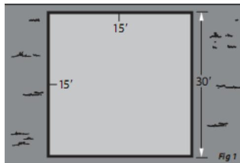
a) Measure and mark the center point on both the length and width of the site (Fig 1 - Overhead View).
