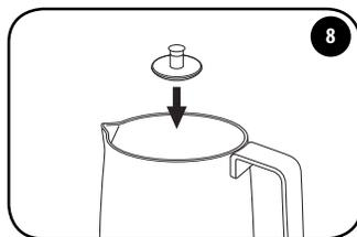
Place the smooth disk for mixing over the pin inside the jug. The smooth disk is housed beneath the motor base.
