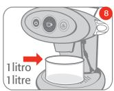
Press the coffee switch O to start the decalcification cycle the coffee switch turns off 5
