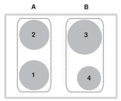
PowerPlus cannot be used for both cooking zones of a group ( $\bf A$  or  $\bf B$ ) at the same time. If PowerPlus is activated for both cooking zones of a group, the power of the cooking zone that was initially set reduces.
