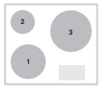
PowerPlus cannot be used in cooking zones 1 and 2 at the same time. If PowerPlus is activated for both cooking zones, the power of the cooking zone that was initially set reduces.
