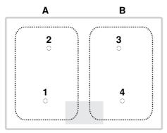
PowerPlus cannot be used for both cooking zones of a group (**A** or **B**) at the same time. If PowerPlus is activated for both cooking zones of a group, the power of the cooking zone that was initially set reduces.
