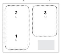
PowerPlus cannot be used in cooking zones 1 and 2 at the same time. If PowerPlus is activated for both cooking zones, the power of the cooking zone that was initially set reduces.
