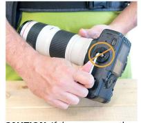
**CAUTION:** if the arrows on the hub are incorrectly aligned during setup, your camera could fall out of your harness.
