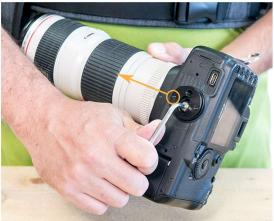
**4.** Now it's time to attach the hub to your camera [using the Allen key provided]. Be sure to align the arrows on the hub in the same direction of the lens.
