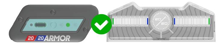
The above left image shows the headgear center light is green, indicating it is connected to a 2020 Armor vest. The vest display on the right shows the two outer lights are green, indicating it is connected to a 2020 Armor headgear.
