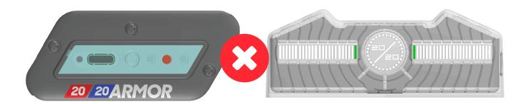
The above left image shows the headgear center light is red, indicating it is not connected to a 2020 Armor vest. The vest display on the right shows the two centre lights are green, and not connected to a headgear.
