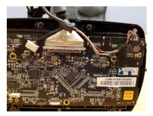
• Using a cutter, cut the area marked with red lines. If not removed, it it will bloct the screw below
