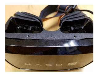
• Be careful not to damage the IR flex cable between the front cover and the unit
