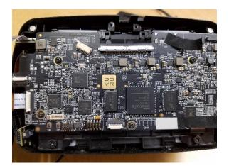
• Carefully remove the main module out of the housing, keep the three screws as you will need them later
