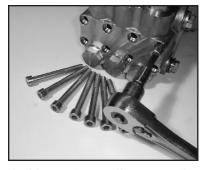
5) Use a 8mm allen wrench to remove the 8 socket head cap screws (34). Carefully slide the valve casing (26) out over the plungers.
