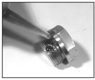
Remove the o-ring (31). Inspect all parts for wear and replace as necessary. Apply one drop of loctite 243 to the valve plugs (32) and tighten to 107 ft.-lbs. (145 NM).
