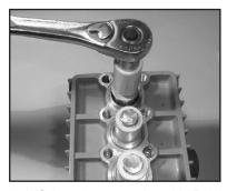
10) If the plunger pipe (16B), is damaged or worn, remove tension screw (16D) and plunger pipe (16B). Check and clean plunger surface (16A) and check flinger (16H). Cover thread of tension screw (16D) with a thin film of Loctite and tighten carefully to 20.7 ft.-lbs. (28 Nm).
