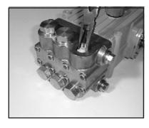
2) Using needle nose pliers, remove the inlet and discharge valve assemblies (27A). Note: It may become neccesary to remove the valve seat (27) from the valve casing using a slidehammer.
