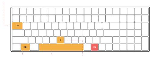
Long Press FN+Win: WinLock Long Press FN+Space: Reset to Default Short Press FN+B: Battery Level Check
