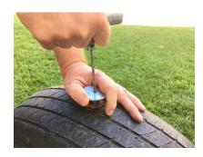
Push the **ring sleeve** down against the tire repair area, and while holding the sleeve firmly against the tire, pull the T-Handle Insertion Tool straight out of the hole until it releases from the tire plug. Cut off the exposed tire plug ends slightly above the tread.
