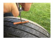
Insert the tire repair string into the hole and push straight down on the insert tool handle until the ends of the tire repair string are sticking out of the tire approximately one-half inch to one inch (13 -25 mm).
