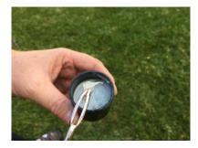
Prepare the Heavy-Duty Steel **T-Handle Insertion Tool** by first dipping the tip into the lubricant.
