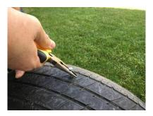
Locate the puncture area and remove the penetrating object.
